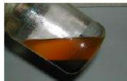
Fig 1. Phase separated fuel from boat tank.
